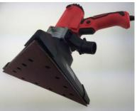
NEVER USE THE SANDING MACHINE WITHOUT APPROPRIATE ABRASIVE PAPER (to prevent serious damage to the work surface).
